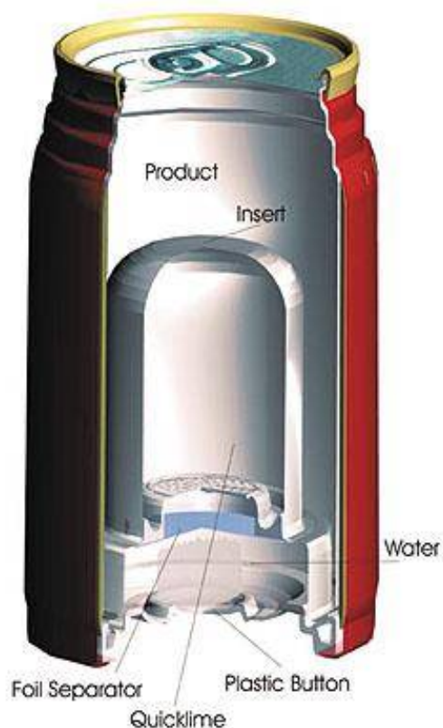
The outside and the inside of the Nestle's "Hot When You Want" coffee can
